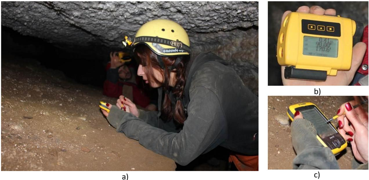
Figure 1. a) Collecting the data with b) LaserAce 1000 rangefinder and c) Juno handheld.
